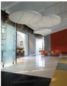
Formations Acoustical Clouds from Armstrong are now available in curved shapes. Designed to enhance acoustics, especially in open plenum spaces, the new line of Formations Curves includes circular, oval, rounded square and rounded rectangle shapes. The unique system consists of ceiling panels with
